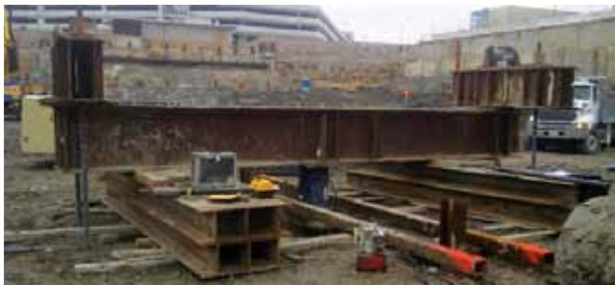
*Test frame for CFA load testing. The CFA pile to be tested is located under the centre of the frame. There are two reaction piles at each end.*
