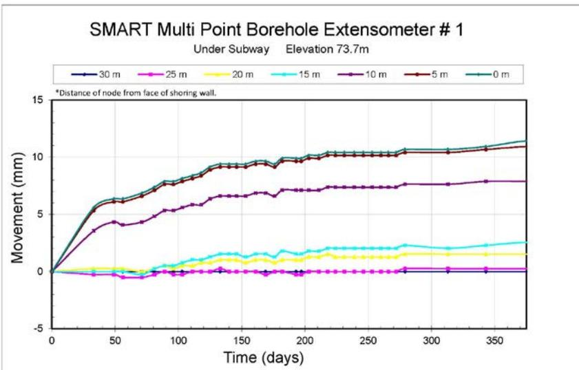
Figure 6: Rock Expansion vs. Time Plot at Subway
