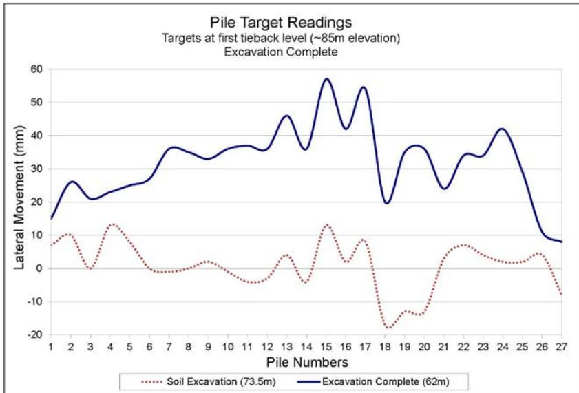
Figure 5: Pile Target Lateral Movement vs. Time
