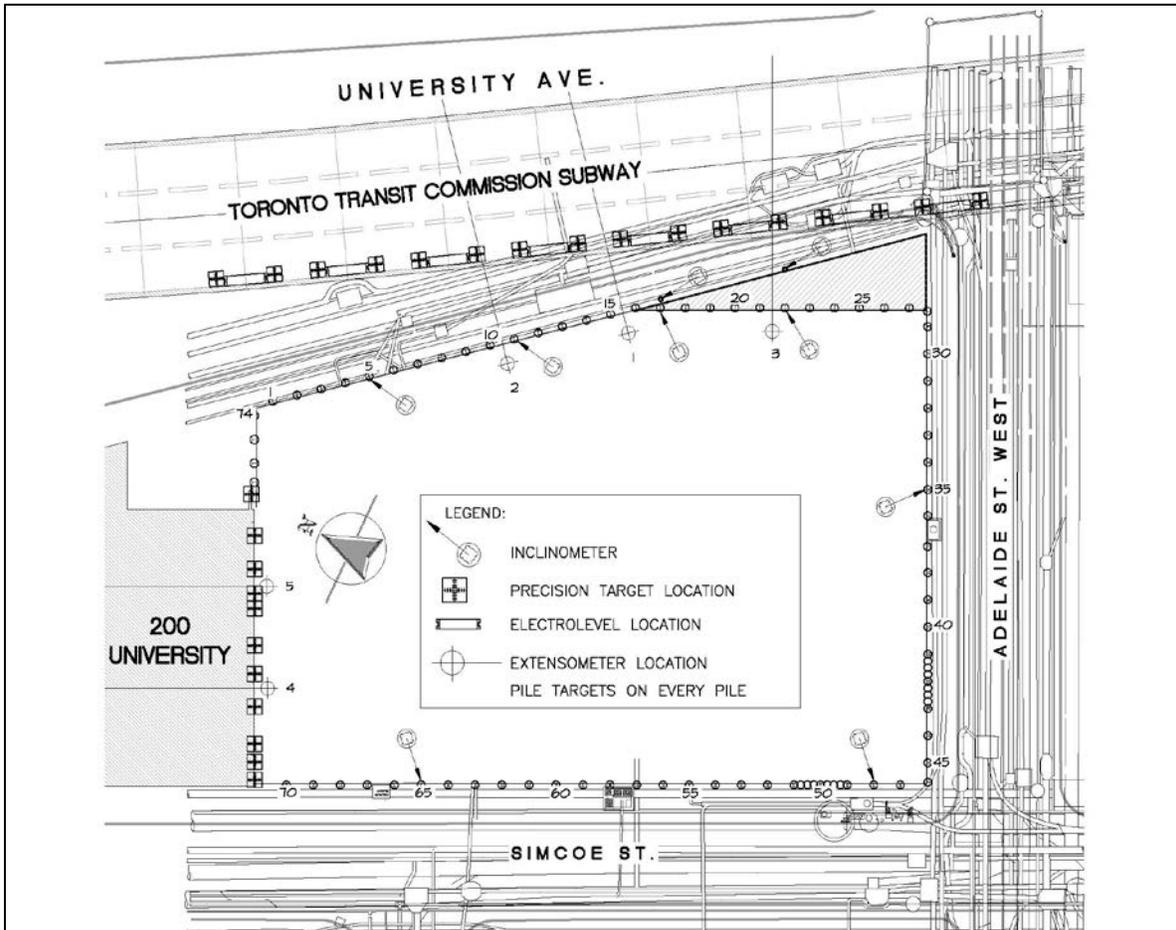
Figure 2: Shoring Layout and Monitoring Plan
