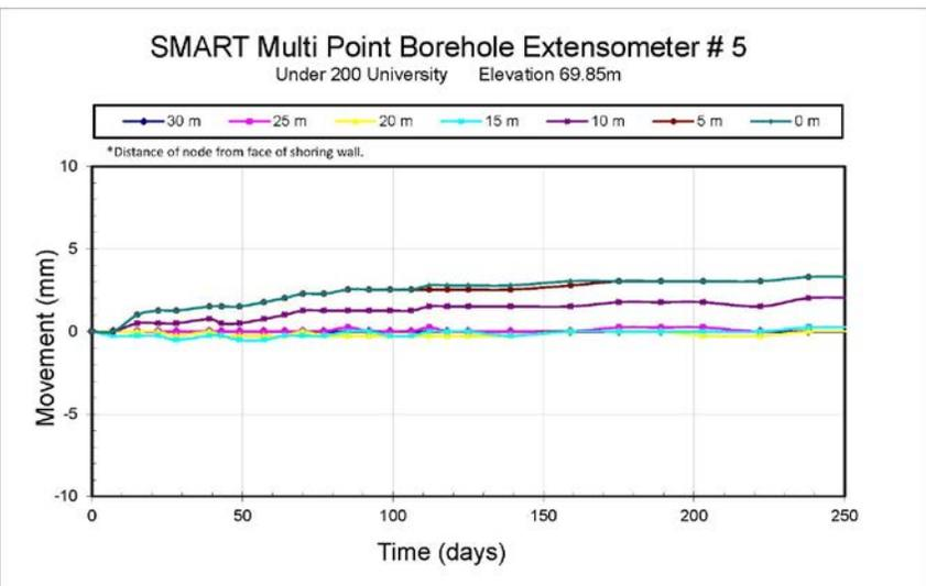
Figure 7: Rock Expansion vs. Time Plot at 200 University
